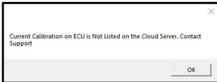
**Reason** → No update is available based on the calibration installed in the ECM or based on the engine serial number entered into the programmer.
