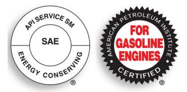
Gasoline engines that are converted for LPG or NG fuels MUST use oils labeled 'FOR GASOLINE ENGINES'. Do not use oils that are specifically formulated for Diesel Engines only. CC or CD classifications oils, even when labeled Heavy Duty or for Natural Gas Engines, ARE NOT ACCEPTABLE.
