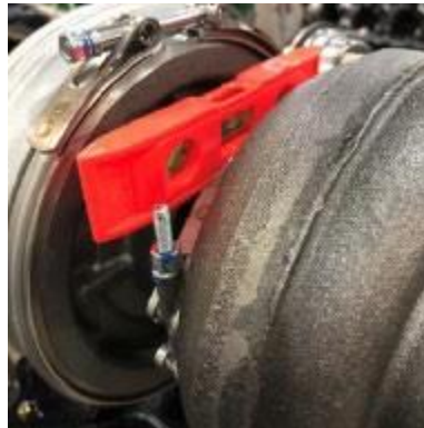
Figure 28. Oil Inlet Leveling
