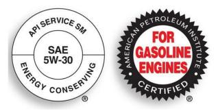
PSI recommends using engine oils that have an API rating of SM or newer. Gasoline engines that are converted for LPG or NG fuels MUST use oils labeled 'FOR GASOLINE ENGINES'. Do not use oils that are specifically formulated for Diesel Engines only. CC or CD classifications oils, even when labeled Heavy Duty or for Natural Gas Engines, **ARE NOT ACCEPTABLE.**
