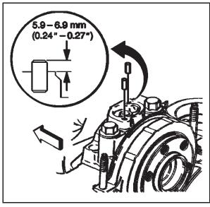
3. Inspect the pins (oil pump locator) for damage and replace the pins if required.
