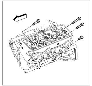
6. Remove the cylinder head bolts and discard.
