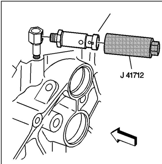
20. If reusing the engine oil pressure gauge sensor, apply PTFE sealant or equivalent to the threads of the engine oil pressure gauge sensor.
