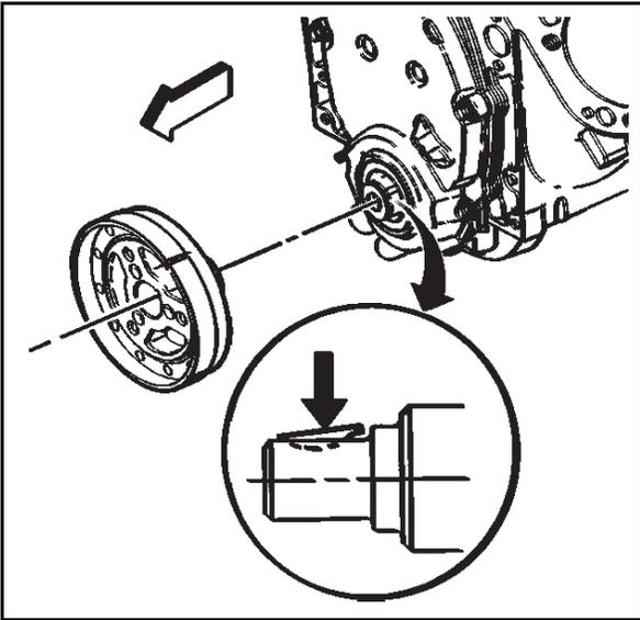
**Notice:** The inertial weight section of the crankshaft balancer is assembled to the hub with a rubber type material. The correct installation procedures (with the proper tool) must be followed or movement of the inertial weight section of the hub will destroy the tuning of the crankshaft balancer.
