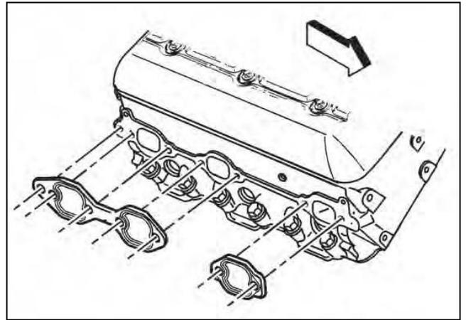
2. Install the exhaust manifold.
