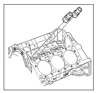
**Important**: Place the valve lifters in the rack in the upright position to maintain the oil inside the valve lifters.
