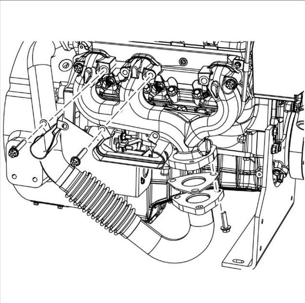
2. Install the exhaust manifold.
