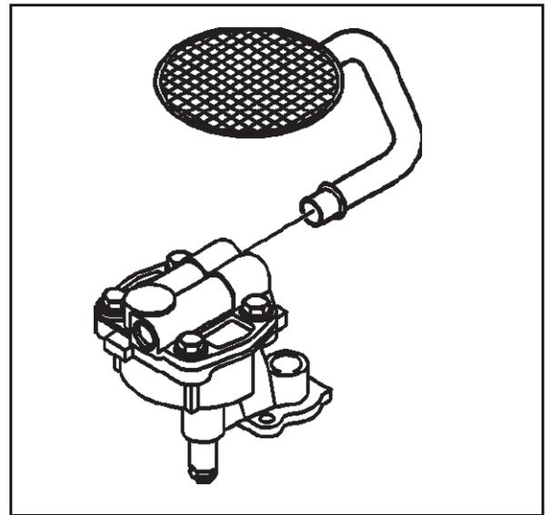
3. Remove the oil pump cover bolts.
