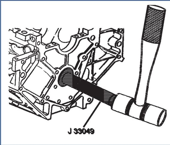
1. Select the handle (10), the expanding driver (4-8), the washer (2 or 3) and the expander assembly (15) from the J 33049.
