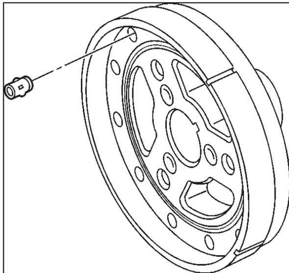
5. Note the position of any front groove pins (crankshaft balancer) (if applicable)
