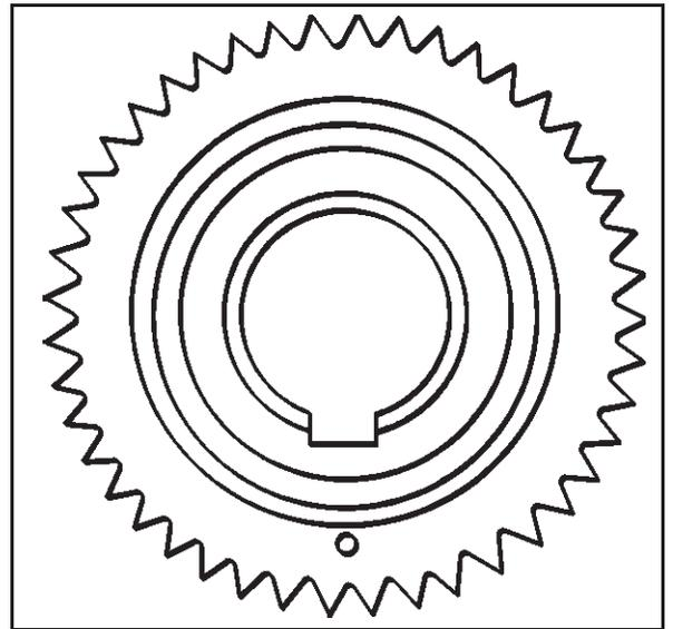
14. Position the balance shaft drive gear onto the engine camshaft.
