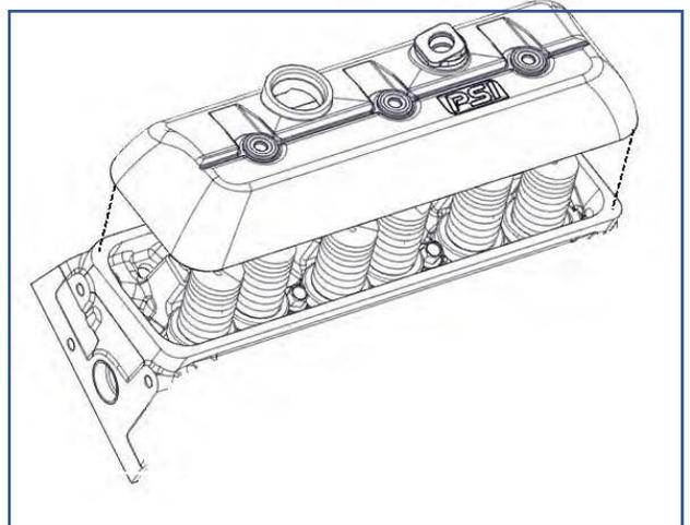
4. Install the valve rocker arm cover bolts.
