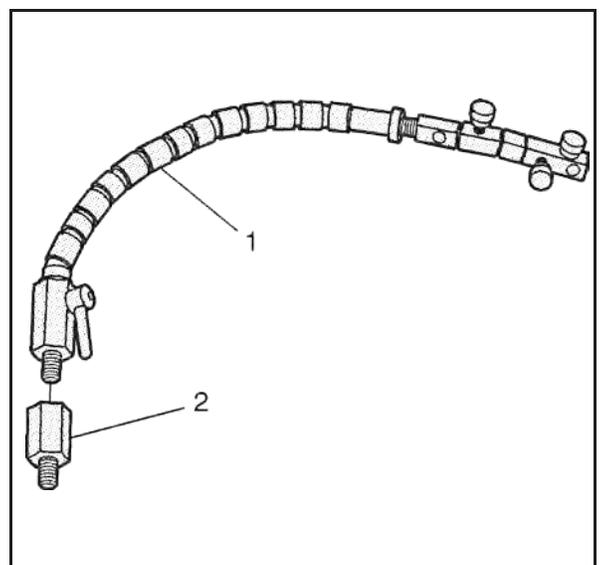
**Important:** The clamp of the swivel base and the shaft of the indicator should be free of oil or other debris. A loose or improperly clamped indicator may indicate incorrect readings.
