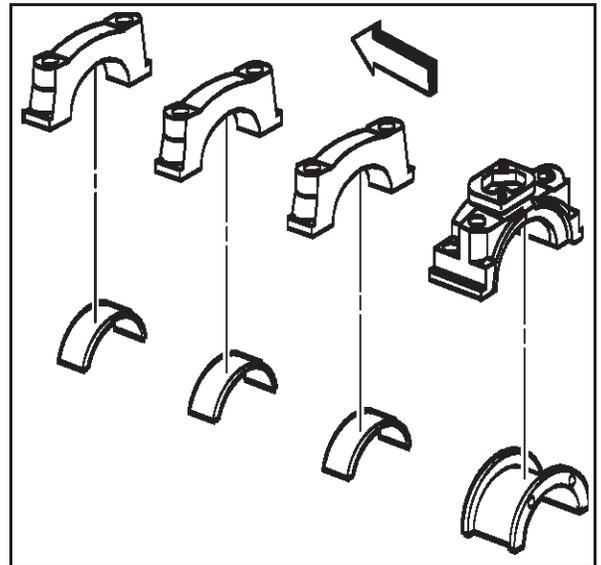
5. Install the crankshaft bearing caps in the original positions and with the arrow on the crankshaft bearing caps in the direction of the front of the engine block.
