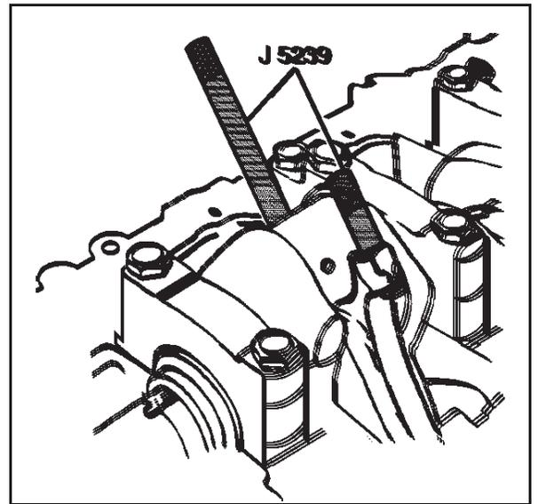
**Important:** Always assemble the connecting rod caps to the matching connecting rods.
