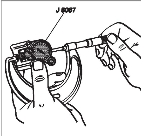
2. Measure the J 8087 with a micrometer and record the reading.
