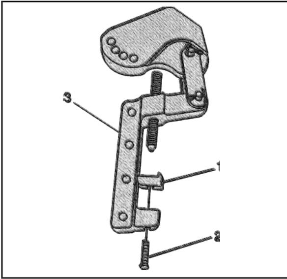
5. Install the foot (1) and bolt (2) to the pivot arm assembly (3). Tighten the bolt until snug.
