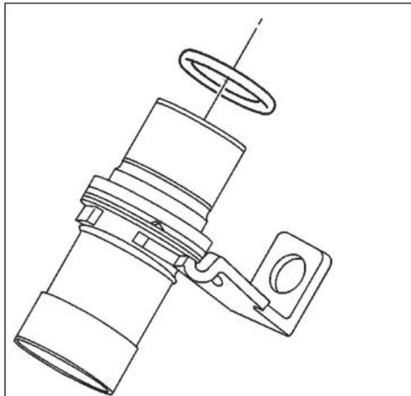
6. Install the crankshaft position sensor until fully seated into the engine front cover.
