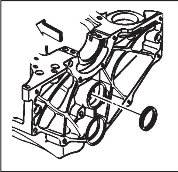
6. Remove the expansion cup plug (camshaft rear bearing hole) and discard.
