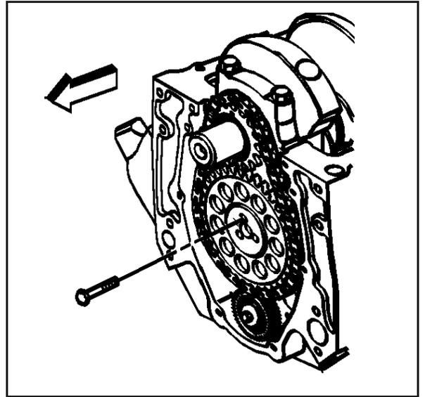
4. Remove the camshaft sprocket and the camshaft timing chain.
