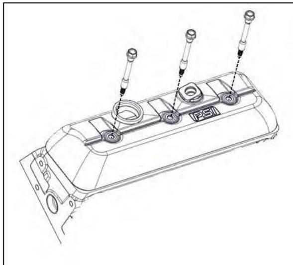
**Valve Rocker Arm Cover Removal (Left) (Distributor Ignition)**
