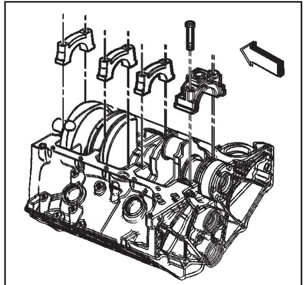
4. Remove the crankshaft.
