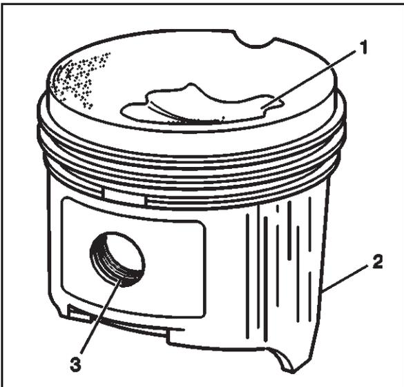
4. Clean the piston oil lubrication holes and slots.
