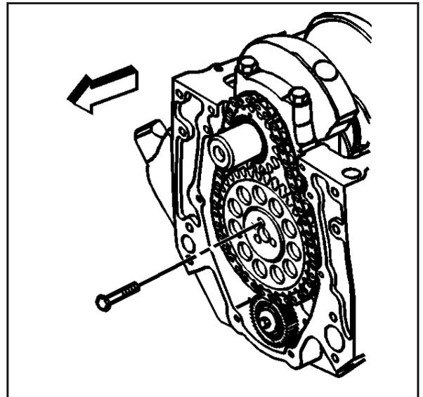
8. Install the crankshaft position sensor reluctor ring.
