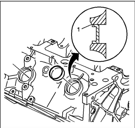
1. Install a NEW oil filter bypass valve.
