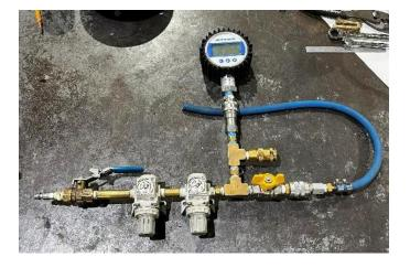
5. Open the pressure regulator valve with the hose connected to the actuator. Ensure the dial indicator is set at 0.
