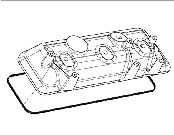
11. Remove the valve rocker arm cover gasket.
