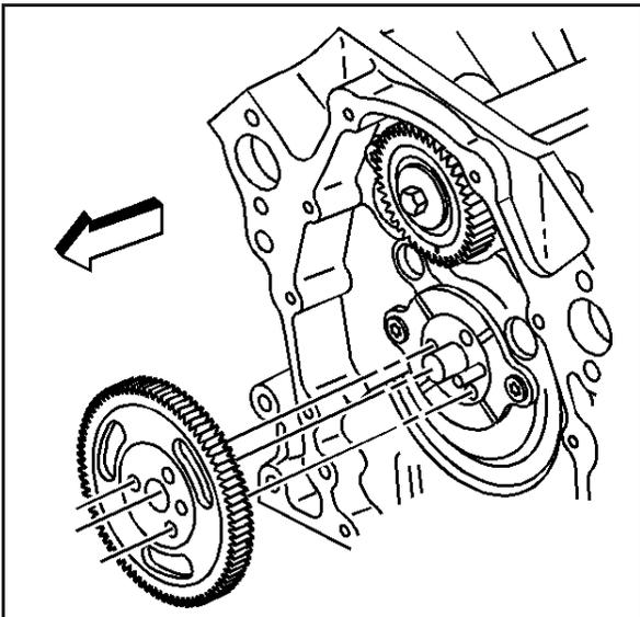
10. Install the balance shaft drive gear. DO NOT install the camshaft sprocket bolts at this time. Apply Clevite Gear Lubricant or equivalent to the Balance Shaft Drive Gear.
