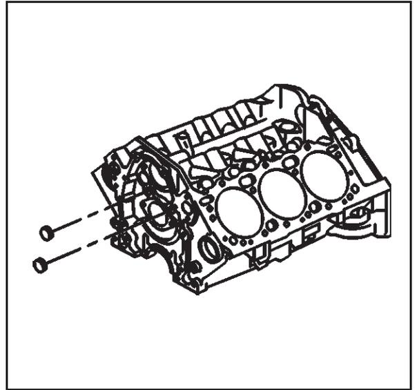
11. Remove the engine block core hole plugs.
