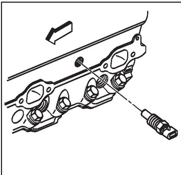
2. Remove the engine coolant temperature gauge sensor (if applicable).
