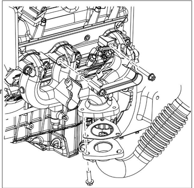
6. Remove and discard the exhaust manifold gaskets.
