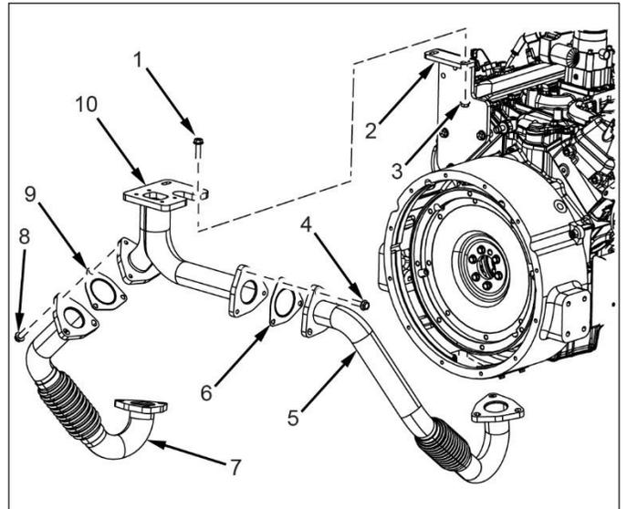
6. Install right side turbo exhaust (3) and new gasket (2) to right side exhaust manifold (1) and secure with bolts (4).
