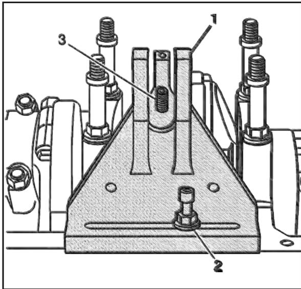
11. Align the center of the base (1) with the screw (3) of the pivot arm assembly. Tighten the bolt (2) until snug.
