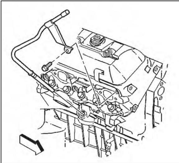
7. Remove the oil level indicator tube bolt.
