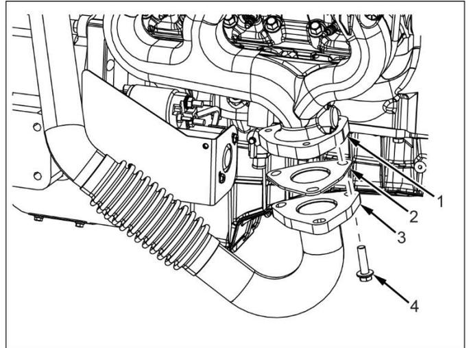
15. Remove bolts (4), right side turbo exhaust (5) and gasket (6) from right side of exhaust Y-Pipe (10). Discard gasket.
