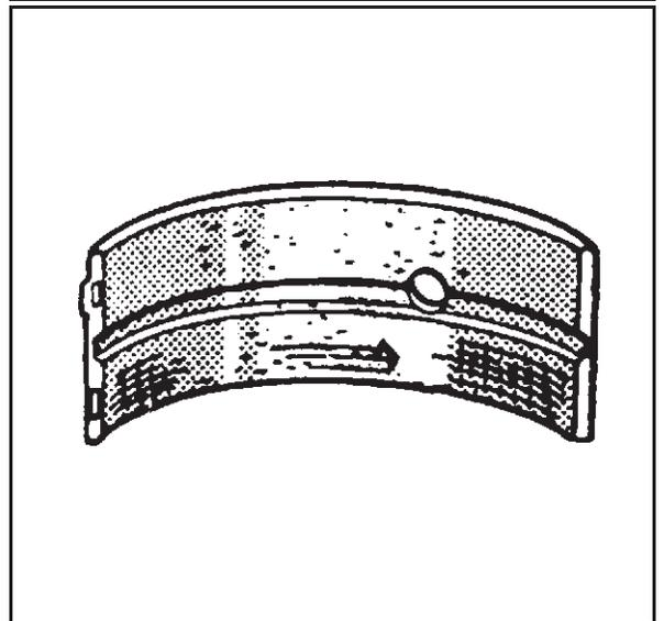
14. Inspect the crankshaft bearings for improper seating indicated by bright, polished sections of the crankshaft bearings.
