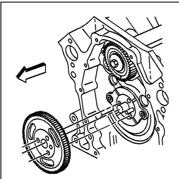
12. Remove the balance shaft drive gear.
