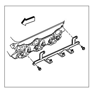
5. Remove the bolts and the spark plug wire support.
