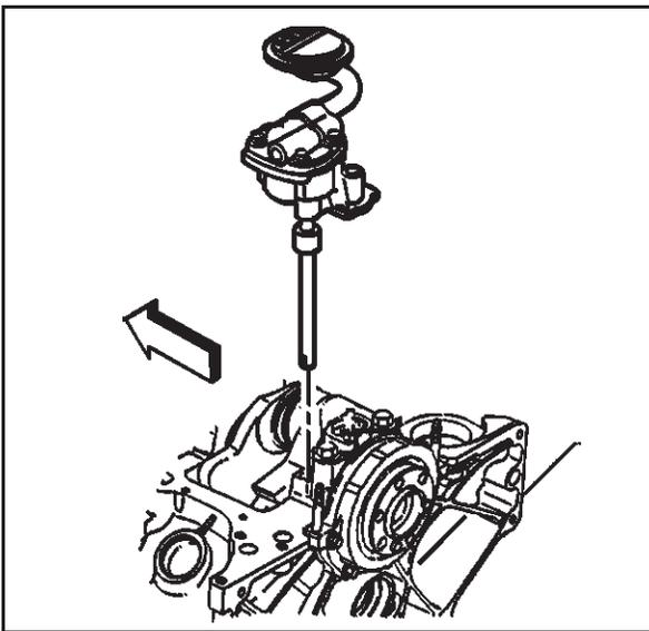
3. Inspect the pins (oil pump locator) for damage and replace the pins if required.
