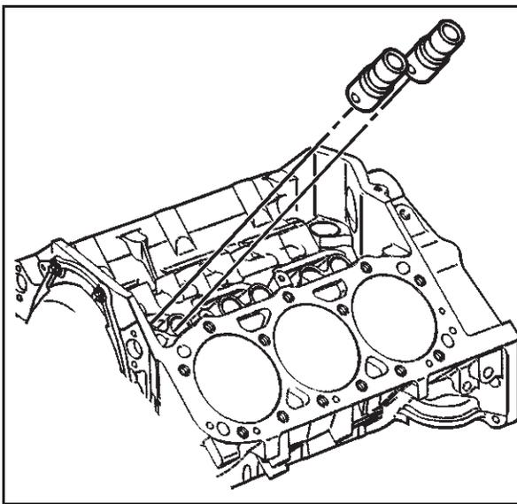
**Valve Lifter Installation**
