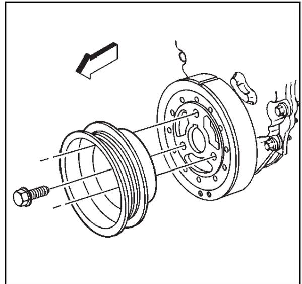
9. Ensure that the crown of the crankshaft balancer washer (2) is facing away from the engine.
