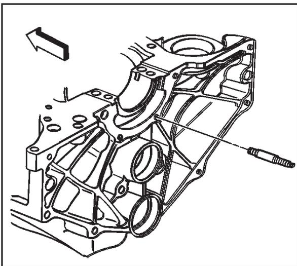
8. Remove the crankshaft rear oil seal housing retainer stud from the engine block.
