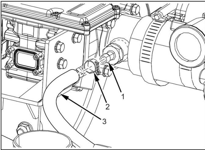
11. Install hose (3) on fitting (1) and slide hose clamp on hose over fitting and secure hose clamp (2).
