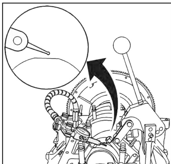
19. The tip of the indicator should be positioned above and NOT in contact with the cap end of the connecting rod.
