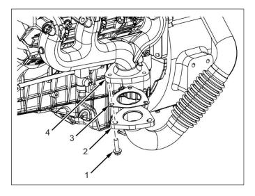
Remove bolts (4), left side turbo exhaust
