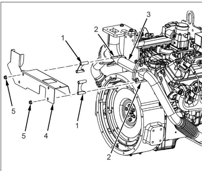
8. Install heat shield (4) and saddles (1) and secure with U-bolts (2) and nuts (5).
