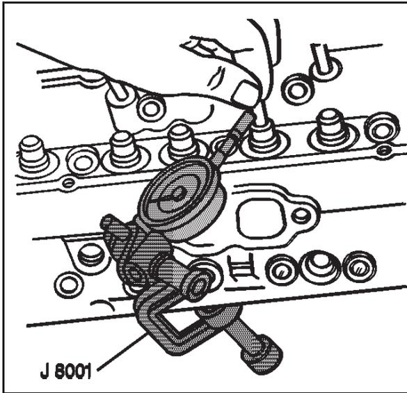
10. Measure the valve stem-to-guide clearance.
