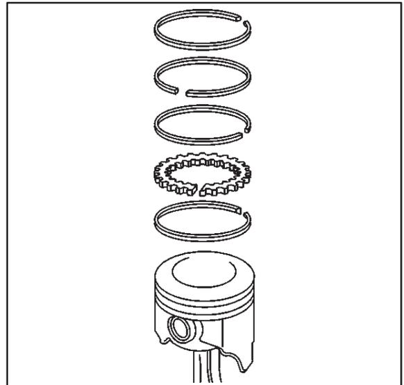
4. Install the J 8037 onto the piston and compress the piston rings.
