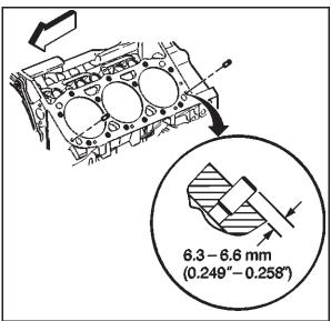
14. Install the left side dowel pins (cylinder head locator.
