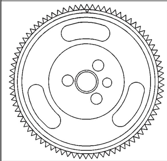
11. Rotate the engine camshaft so that the timing mark on the balance shaft drive gear is in the 12 o'clock position.
