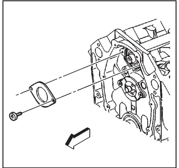
**Important:** The balance shaft and the balance shaft front bearing are serviced only as a package. Do not remove the balance shaft front bearing from the balance shaft.
