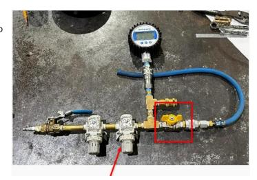
Gradually increase the pressure applied to the hose while observing the dial indicator. Record the pressure value (psig) at the point where the dial indicator shows exactly 3mm of actuator rod travel.
