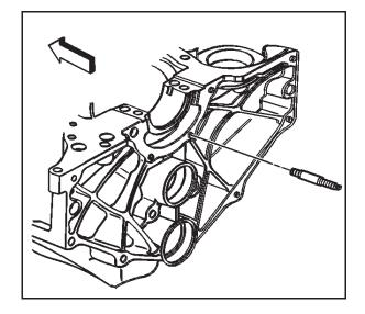
8. Remove the crankshaft rear oil seal housing retainer stud from the engine block.
