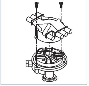
Install the distributor cap and NEW distributor cap bolts.
