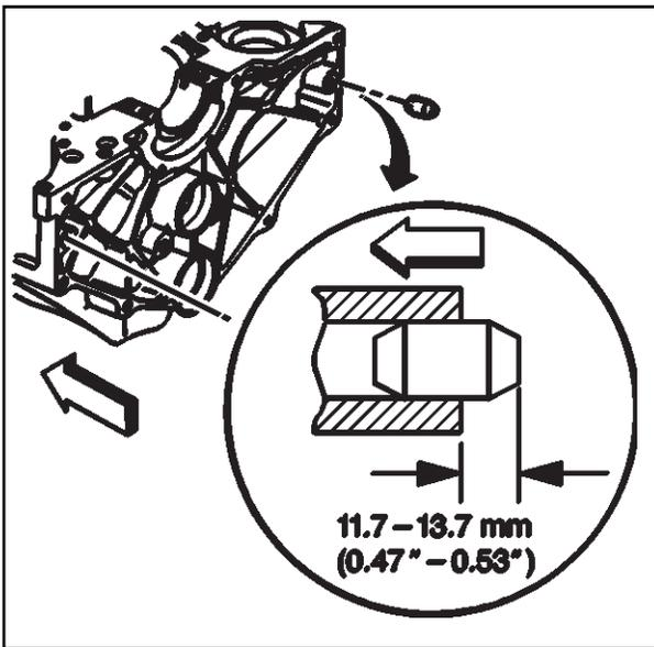
13. Install the dowel straight pins (if required). Ensure tapered end is facing outward.
