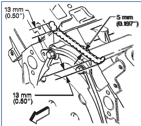
**Notice:** Care must be used to apply the correct amount of sealant onto the gaskets. Applying excessive amounts of sealant may prohibit the intake manifold gaskets from sealing properly.
