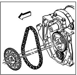
4. Rotate the crankshaft until the crankshaft sprocket is at the 12 o'clock position.
