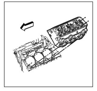
*Notice:* After removal, place the cylinder head on two wood blocks to prevent damage.
