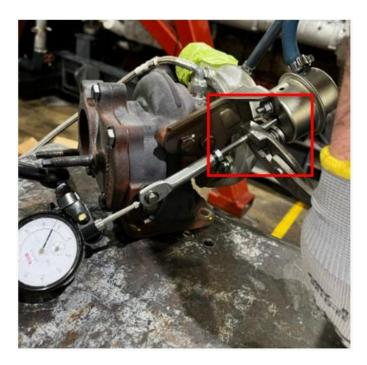
To adjust the wastegate pressure, rotate the actuator rod with pliers as needed. For increased pressure, turn the rod clockwise 1-2 rotations; for decreased pressure, turn it counterclockwise 1-2 rotations. Make adjustments incrementally to achieve the desired setting.
