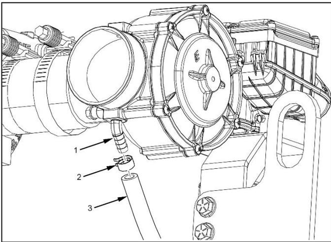
12. Install hose (3) on fitting (1) and slide hose clamp on hose over fitting and secure hose clamp (2).
