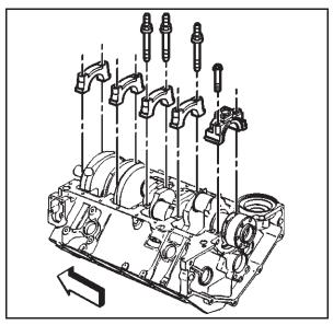
Insert a piece of paper card stock onto the crankshaft journal. Install the bearing half, bearing cap and bolts. Refer to Fastener Tightening Specifications.
