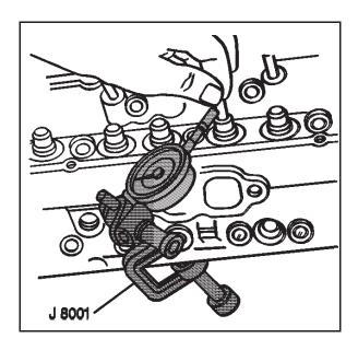
10. Measure the valve stem-to-guide clearance.
