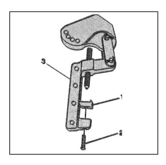
5. Install the foot (1) and bolt (2) to the pivot arm assembly (3). Tighten the bolt until snug.
