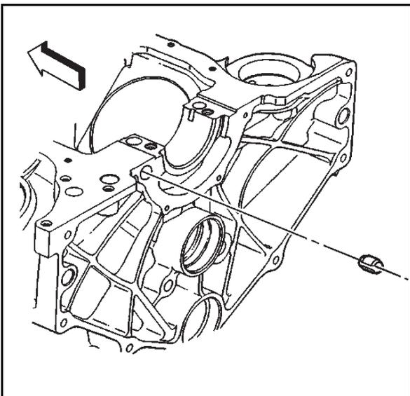
8. Remove the spring type S pin (crankshaft rear oil seal housing locator) (if required).
