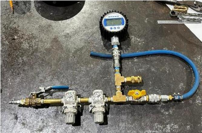
5. Open the pressure regulator valve with the hose connected to the actuator. Ensure the dial indicator is set at 0.
