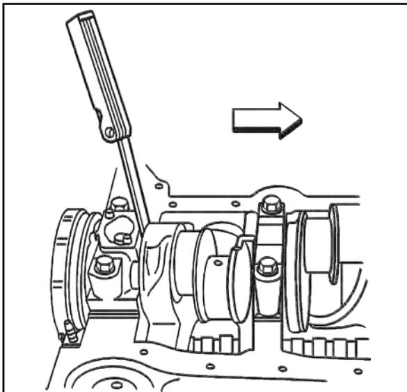
8. Use a suitable support to support the crankshaft on the front and rear journals.
