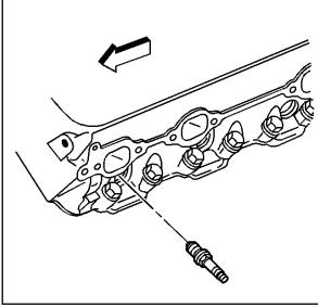
4. Remove the bolts and the spark plug wire support.
