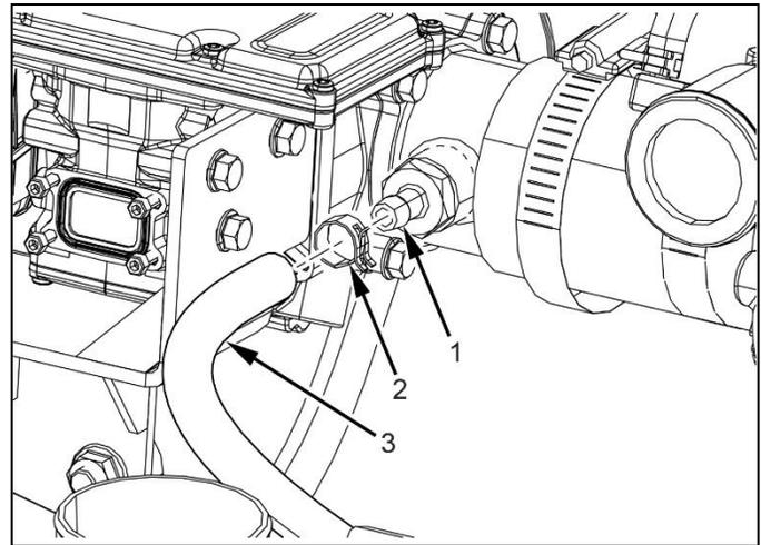
3. Loosen clamp (1) and slide back on hose (2).
