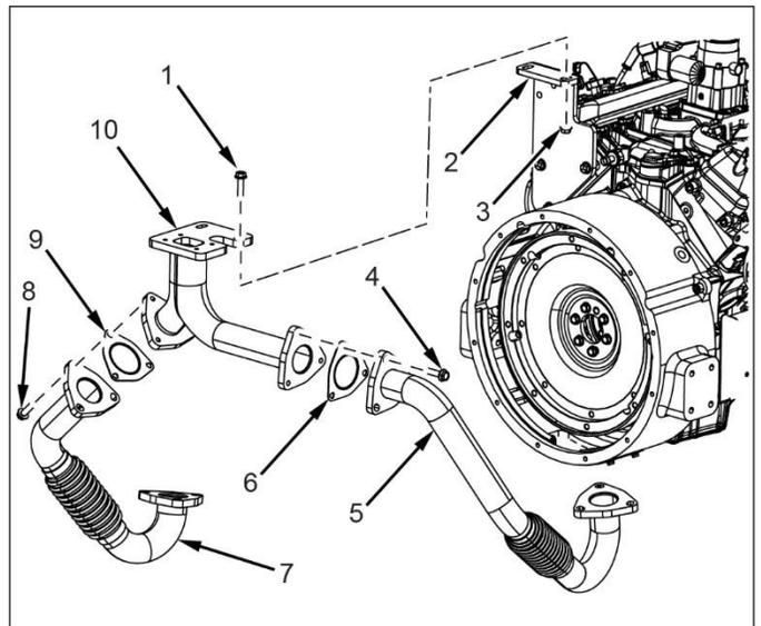
18. Remove bolts (3), turbo mounting bracket (1) and spacers (2) securing from engine.
