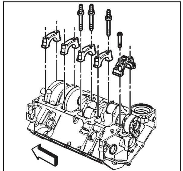
4. Insert a piece of paper card stock onto the crankshaft journal. Install the bearing half, bearing cap and bolts. Refer to *Fastener Tightening Specifications*.
