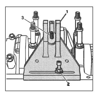
11. Align the center of the base (1) with the screw (3) of the pivot arm assembly. Tighten the bolt (2) until snug.
