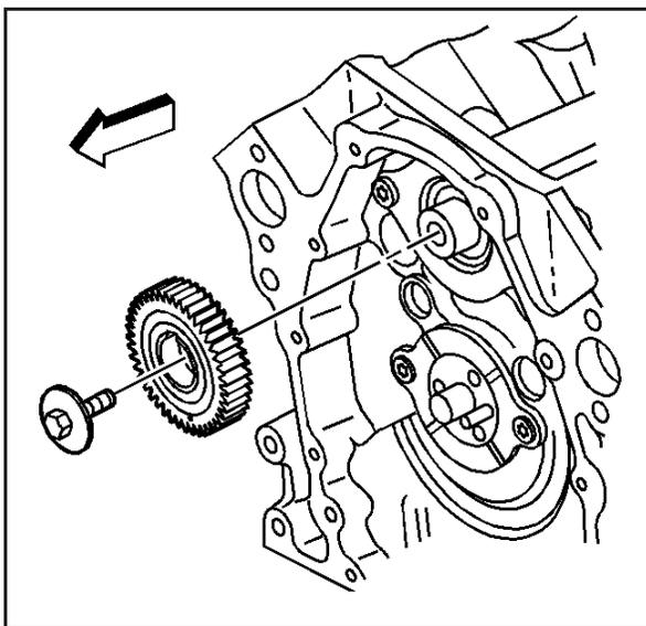
**Important:** The balance shaft drive and balance shaft driven gears are serviced as a set. The set includes the balance shaft driven gear bolt.
