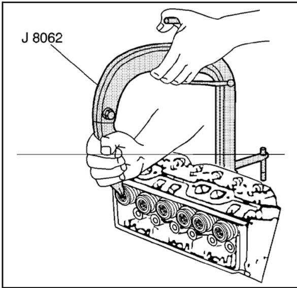
**Caution:** Compressed valve springs have high tension against the valve spring compressor. Valve springs that are not properly compressed by or released from the valve spring compressor can be ejected from the valve spring compressor with intense force. Use care when compressing or releasing the valve spring with the valve spring compressor and when removing or installing the valve stem keys. Failing to use care may cause personal injury.
