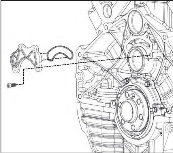
11. Clean all debris from crossover plate and seal. Also clean all debris from engine block before installing crossover plate.
