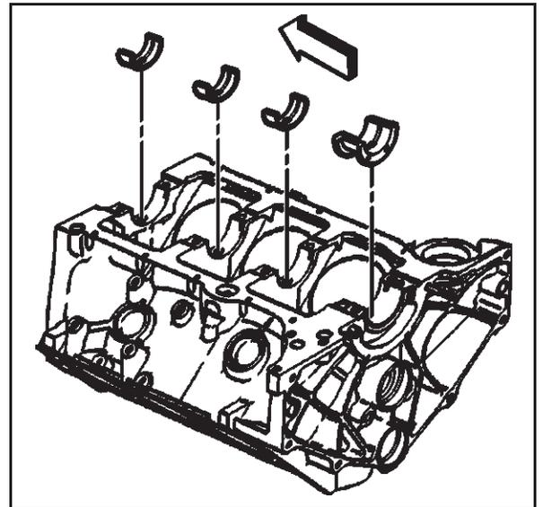
4. Install the bearing cap bolts and tighten to specifications.
