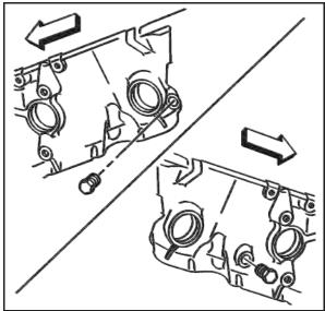
17. If reusing the engine oil pressure sensor fitting, apply PTFE sealant or equivalent to the threads of the engine oil pressure sensor fitting.
