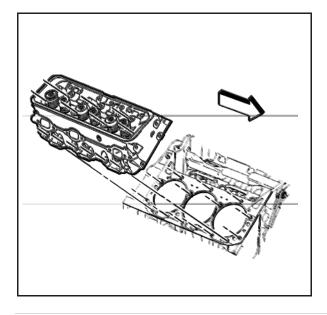
5. Install the cylinder head onto the engine block.
