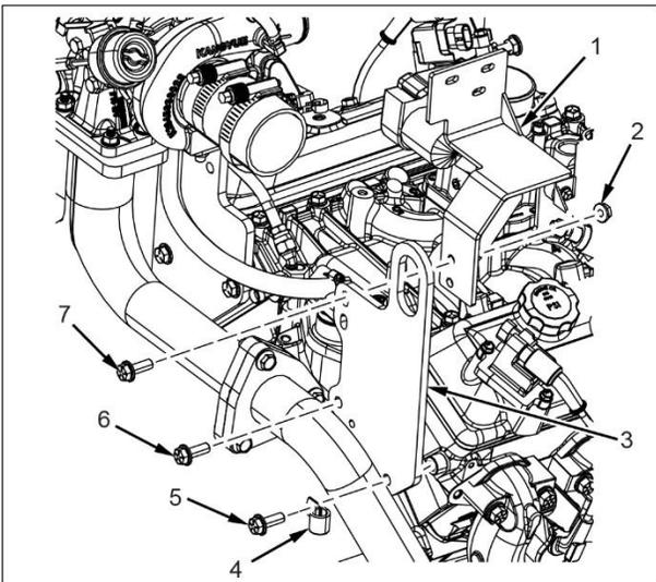
6. Remove nuts (2) and bolts (7) from EPR bracket (1) and rear lifting bracket (3). Remove EPR bracket (1).
