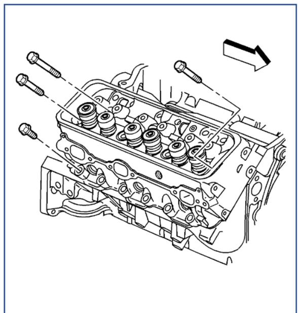
**Notice:** After removal, place the cylinder head on two wood blocks to prevent damage.
