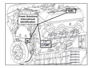
The engine serial number is located on the valve cover of the engine as well as stamped into the left rear of the engine block. The engine serial number format is shown below. 4.3P or 43P followed by a sequence of numbers.
