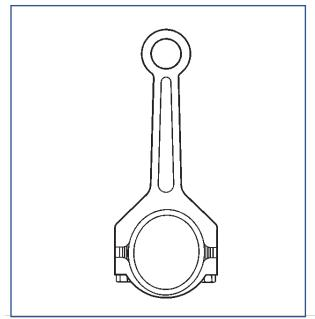
16. Inspect the connecting rod for an out-of-round bearing bore. Refer to *Engine Mechanical Specifications*.
