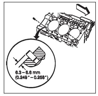
**Important:** Do not use any type of sealer on the cylinder head gasket (unless specified).
