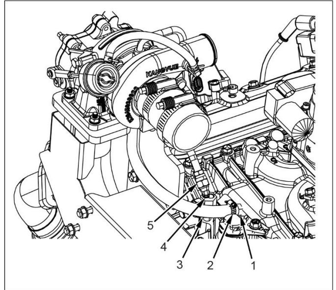
5. Remove nuts (2) securing the turbocharger (1) to the exhaust Y-Pipe (5). Discard nuts.
