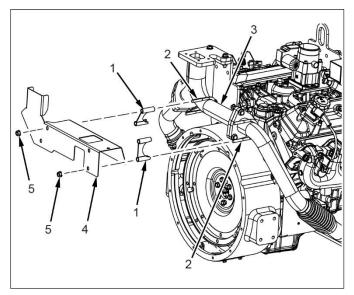
8. Install heat shield (4) and saddles (1) and secure with U-bolts (2) and nuts (5).
