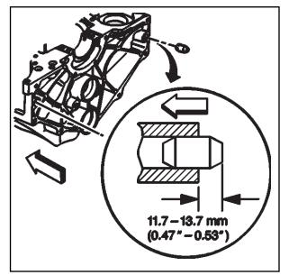
13. Install the dowel straight pins (if required). Ensure tapered end is facing outward.
