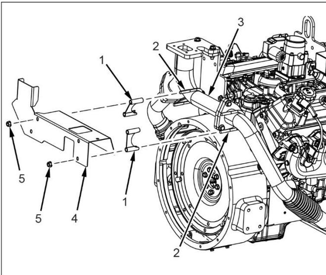
12. Remove nuts (5), heat shield (4), saddles (1) and U-bolts (2) from exhaust pipe (5).
