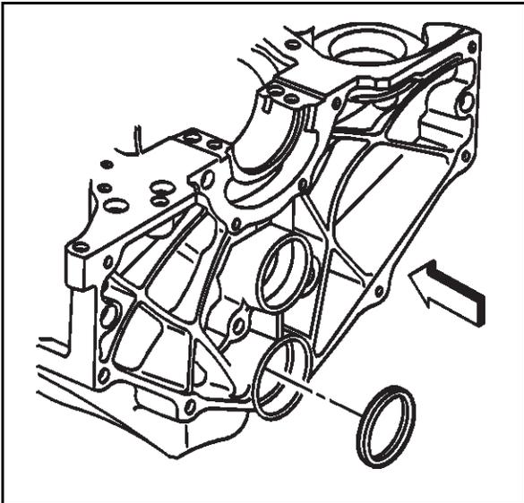
7. Remove the expansion cup plug (balance shaft rear bearing hole) and discard.
