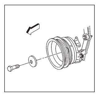
10. Install the crankshaft balancer washer and the bolt.
