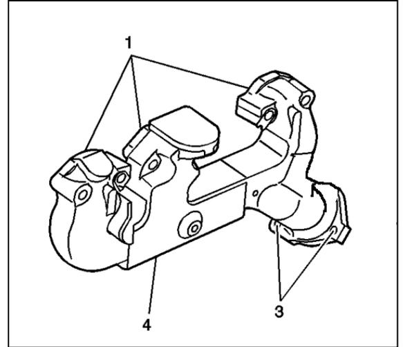
4. Measure the alignment or surface flatness of the exhaust manifold flanges using a straight edge and a feeler gauge. Refer to *Engine Mechanical Specifications*.
