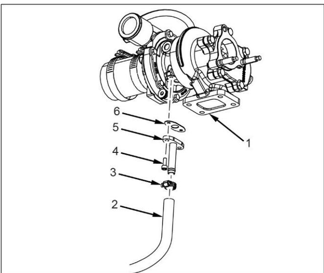
9. Install fitting and new gasket (6) to turbocharger (1) with screws (4).
