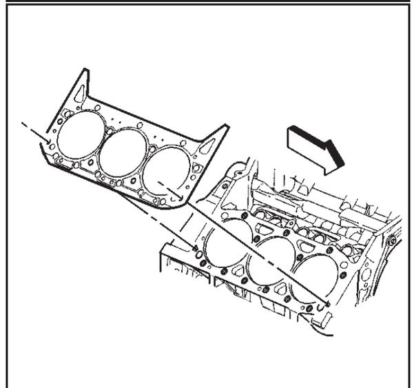
6. Remove the dowel pins (cylinder head locator) (if required).
