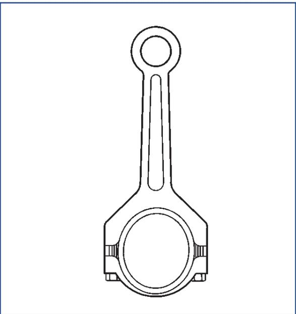
16. Inspect the connecting rod for an out-of-round bearing bore. Refer to *Engine Mechanical Specifications*.
