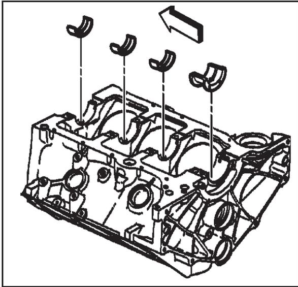
6. Remove the crankshaft bearings from the engine block.
