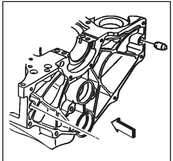
4. Remove the engine block left side oil gallery plug.
