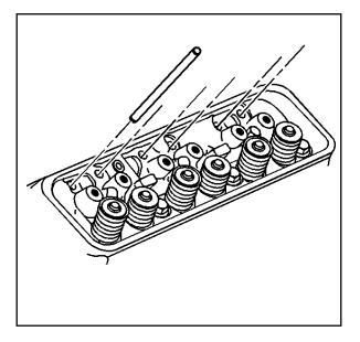
2. Remove the valve pushrods.
