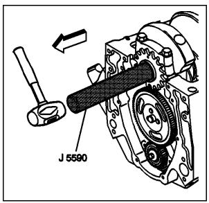
2. Align the keyway of the crankshaft sprocket with the crankshaft balancer key.
