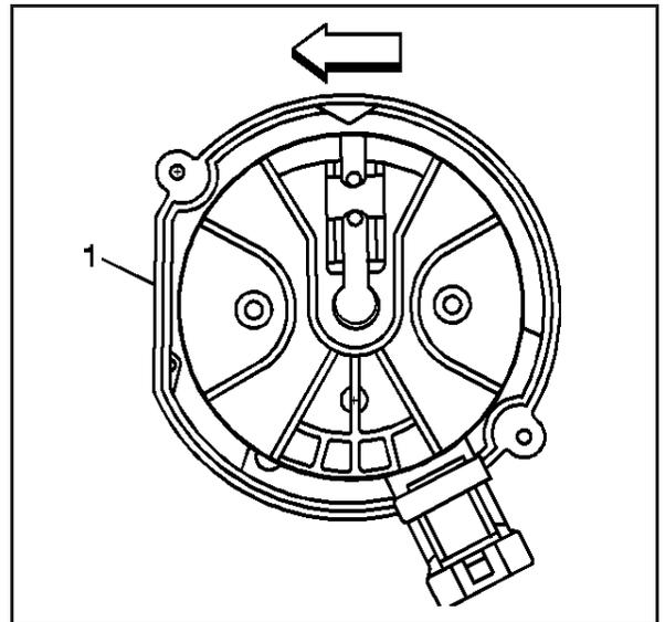
8. Install the distributor and distributor clamp.
