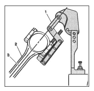
12. Align the link (1) of the pivot arm assembly on a plane (3) equal to that of the connecting rod beam (2).
