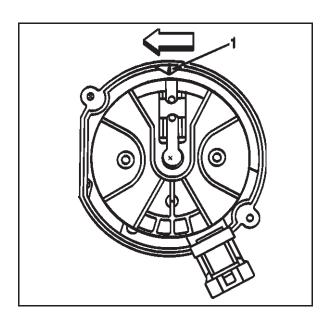
9. Once the distributor is fully seated, align the distributor rotor segment with the number 6 pointer (1) that is cast into the distributor base.
