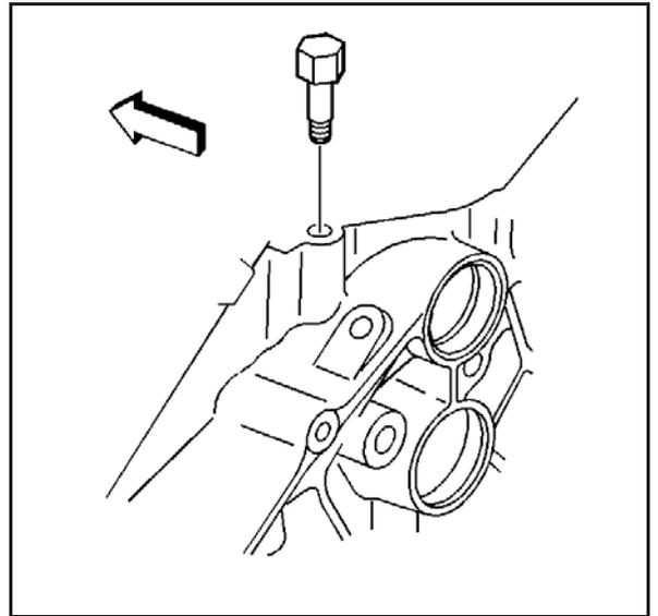
3. Remove the dowel straight pins
