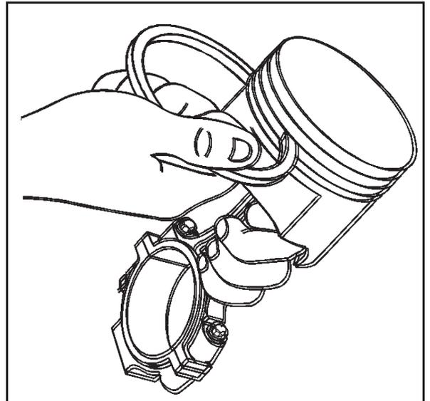
8. Measure the piston ring side clearance with a feeler gauge.
