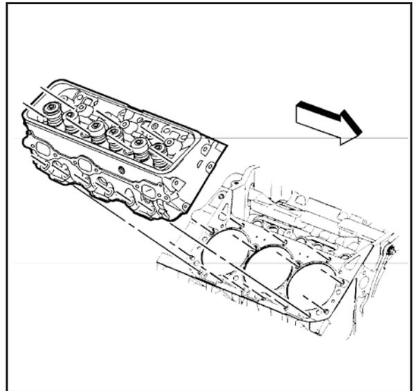
5. Remove and discard the cylinder head gasket.
