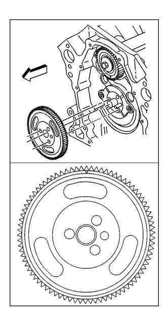
10. Install the balance shaft drive gear. DO NOT install the camshaft sprocket bolts at this time. Apply Clevite Gear Lubricant or equivalent to the Balance Shaft Drive Gear.
