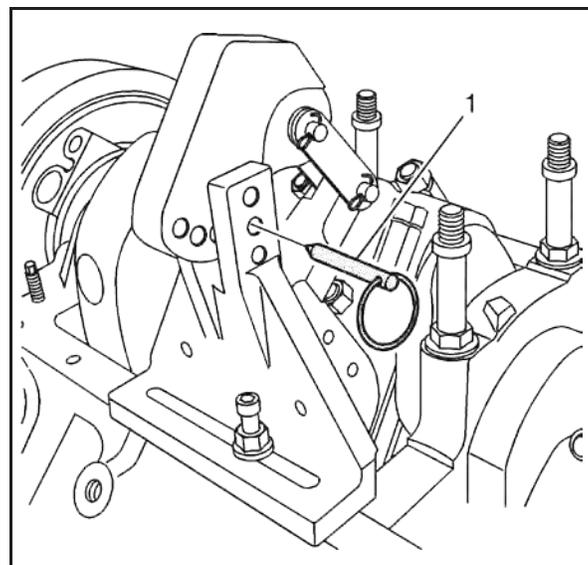
13. With the link of the pivot arm assembly aligned to the beam of the connecting rod, position the pivot arm to the base and insert the pin (1).
