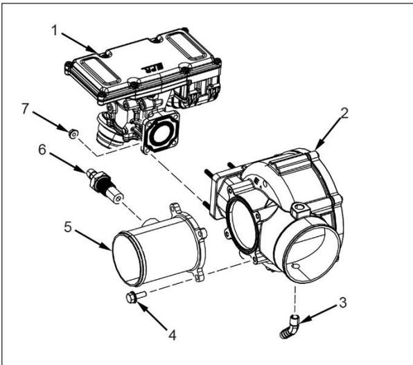
2. Remove the nuts (7) securing regulator (1) to mixer (2). Remove regulator (1) from mixer (2).
