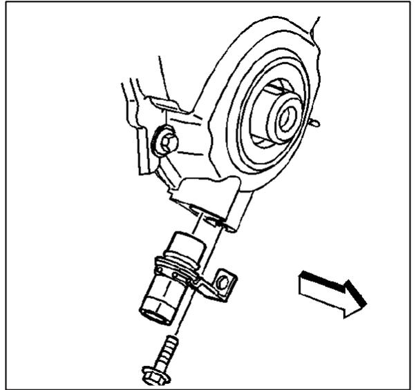
3. Remove the crankshaft position sensor seal (O-ring).
