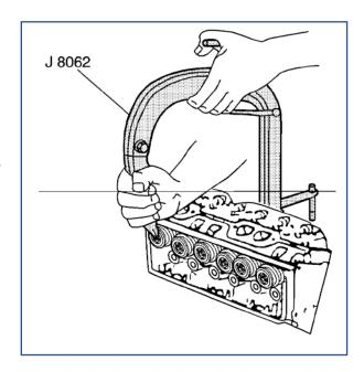
**Important:** Mark, sort and organize the components so that the components can be reinstalled in their original location and position.
