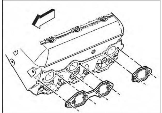
2. Install the exhaust manifold.
