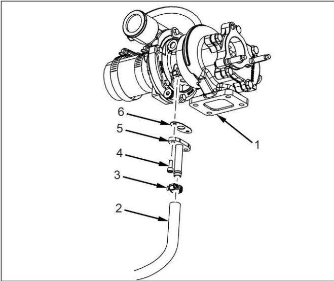
10. Loosen hose clamp (3) on oil return line (2) and slide back on hose. Remove oil return line (2) from fitting (5).
