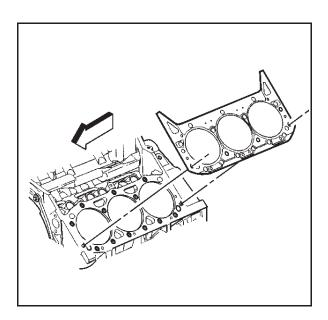
9. Remove the dowel pins (cylinder head locator) (if required).
