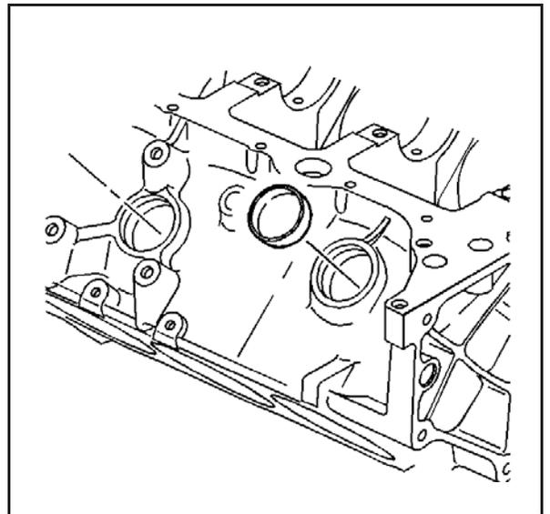
12. Remove the oil filter bypass valve and discard.
