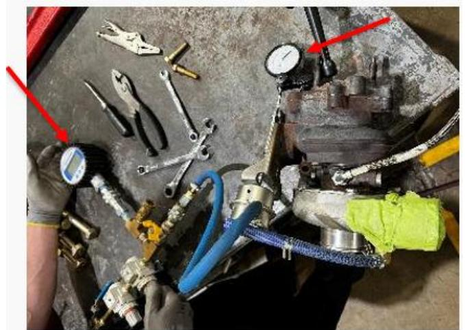
7. The initial pressure observed represents the current setting of the wastegate actuator. To make adjustments, release the pressure to allow the actuator arm to return to its original position.
