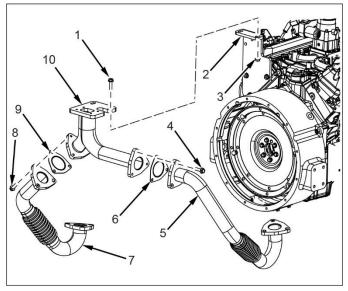
18. Remove bolts (3), turbo mounting bracket (1) and spacers () securing from engine.
