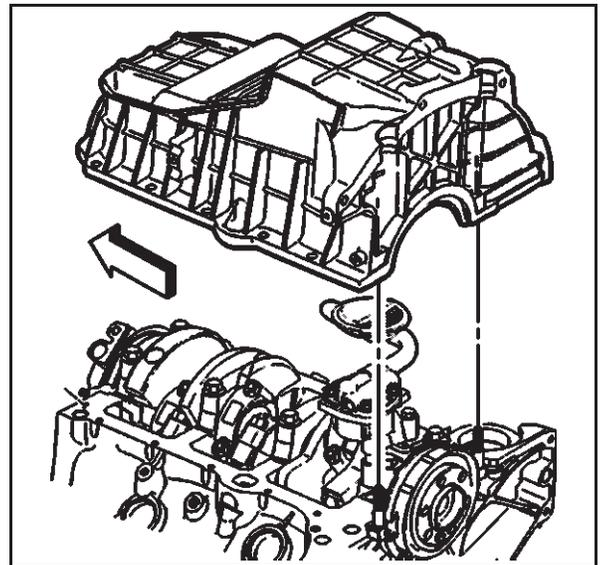
1. Remove the oil pan gasket.
