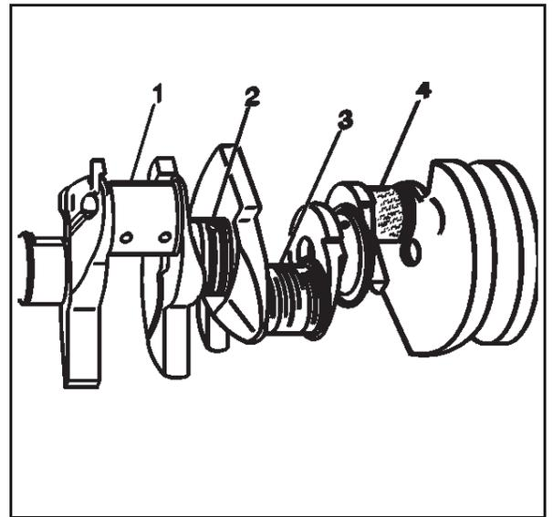
6. Inspect the crankshaft balancer key (1), the keyway (2) and the threaded hole (3) for damage.
