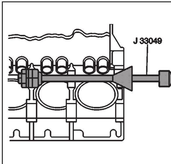
**Important:** A loose camshaft bearing may be caused by an enlarged, out-of-round, or damaged engine block camshaft bearing bore.
