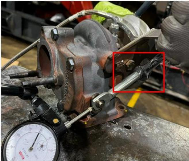
10. After making adjustments, tighten the rod nut and torque it to 12-14 Nm (approximately 8.9-10.3 ft-lbs).
