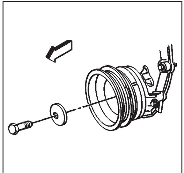
2. Remove the bolts and the crankshaft pulley.
