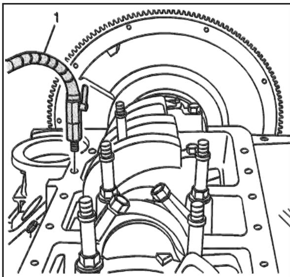
17. Install the swivel base (1) to the oil pan rail of the engine block. Tighten until snug.
