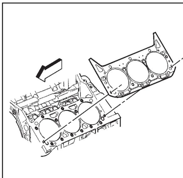
9. Remove the dowel pins (cylinder head locator) (if required).
