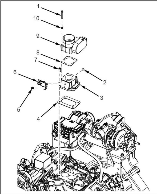
1. Install adapter (3), new gasket (4), apply blue loctite to threads of screws and install screws (7) on intake manifold.
