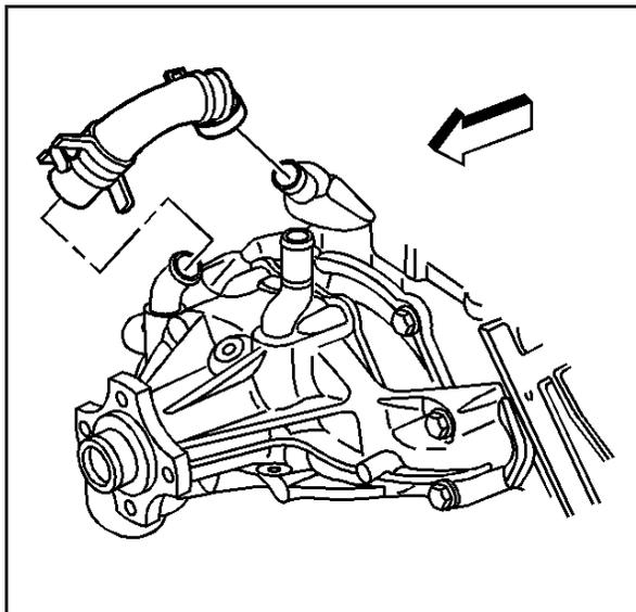
2. Remove the clamps and water pump inlet hose.
