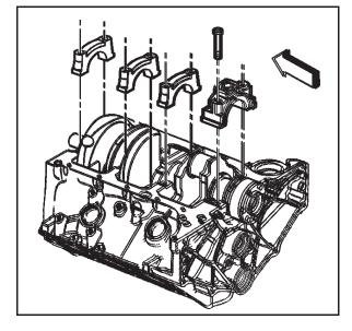
4. Remove the crankshaft.
