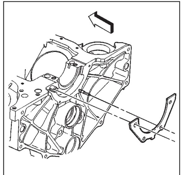
3. Install the crankshaft rear oil seal housing onto the crankshaft rear oil seal housing retainer stud.
