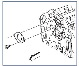
Install the balance shaft driven gear onto the balance shaft.
