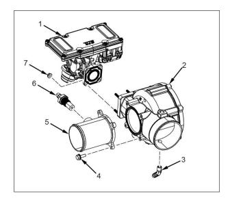
8. Install the regulator Assy onto the hose (2). Leave clamp loose at this time.
