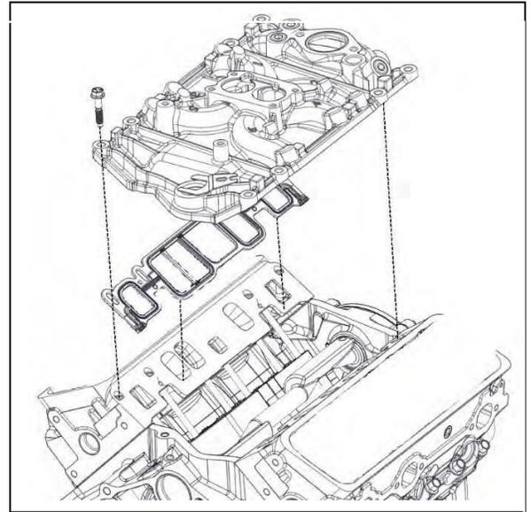
**Notice:** Proper lower intake manifold fastener tightening sequence and torque is critical. Always follow the tightening sequence and torque the intake manifold bolts using the 3-step method. Failing to do so may distort the crankshaft bearing bore alignment and cause damage to the crankshaft bearings.
