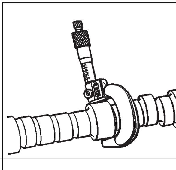
8. Measure for a bent engine camshaft or excessive engine camshaft runout using the J 7872.
