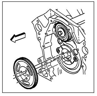
12. Remove the balance shaft drive gear.
