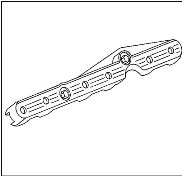
4. Inspect the valve lifter pushrod guides for excessive wear.
