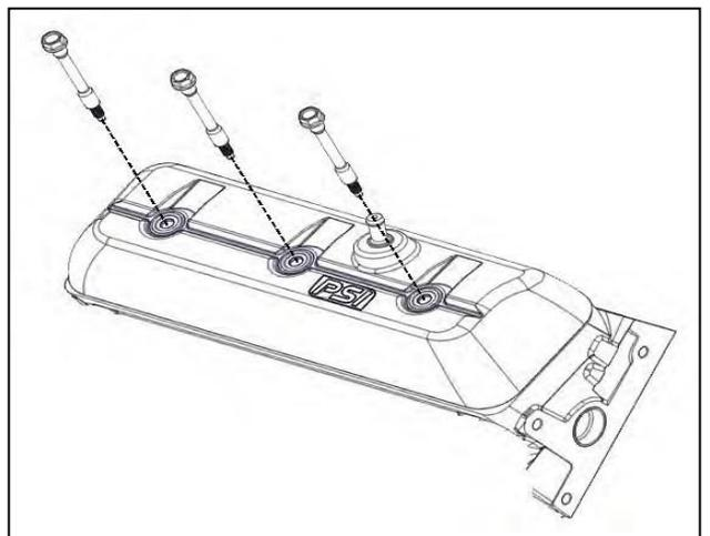
4. Remove the valve rocker arm cover.
