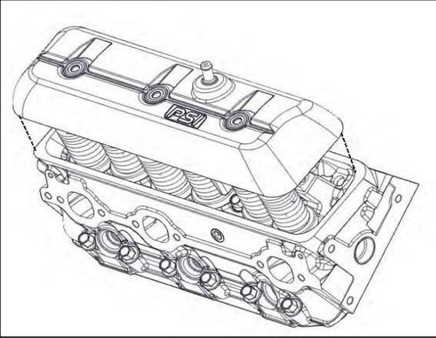
5. Remove the valve rocker arm cover gasket.
