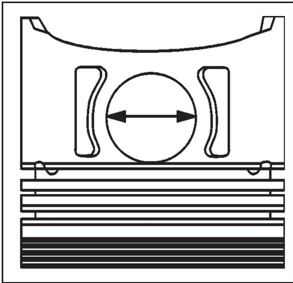
13. To determine piston pin-to-bore clearance, use an inside micrometer and measure the piston pin bore.
