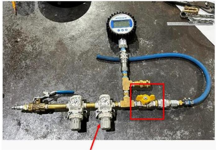
6. Gradually increase the pressure applied to the hose while observing the dial indicator. Record the pressure value (psig) at the point where the dial indicator shows exactly 3mm of actuator rod travel.
