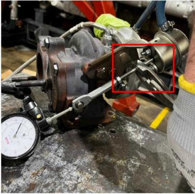
9. To adjust the wastegate pressure, rotate the actuator rod with pliers as needed. For increased pressure, turn the rod clockwise 1-2 rotations; for decreased pressure, turn it counterclockwise 1-2 rotations. Make adjustments incrementally to achieve the desired setting.
