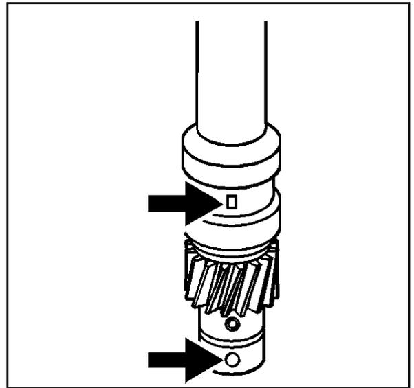
6. Align the slotted tang in the oil pump driveshaft with the distributor driveshaft.
