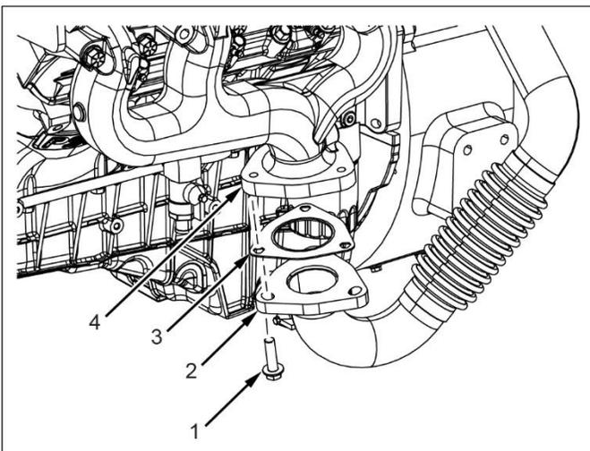
13. Remove bolts (4), left side turbo exhaust (3) and gasket (2) from left side exhaust manifold (1). Discard gasket.
