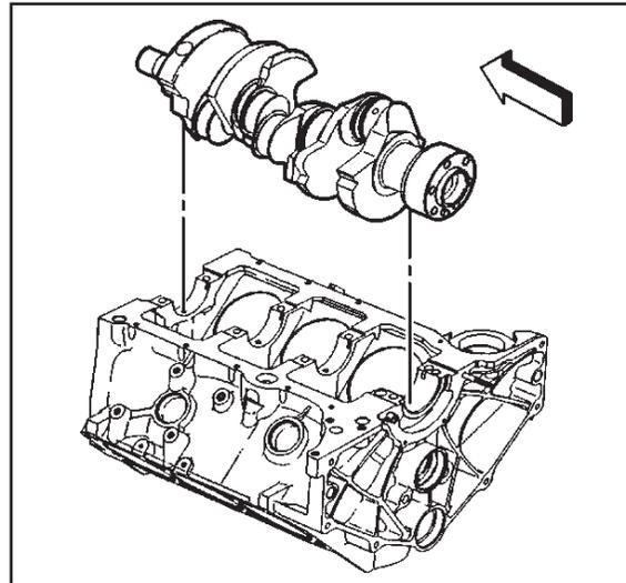
5. Install the crankshaft bearings into the crankshaft bearing caps. Align the tang on the bearing to the keyway in the main caps. Be sure the bearing is flat along the top the main cap. Apply engine assembly lubricant to the bearings in the main cap bearings.
