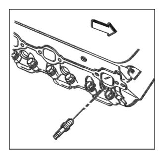
14. Measure the NEW spark plugs for the proper gap. Adjust the spark plug gap if necessary.
