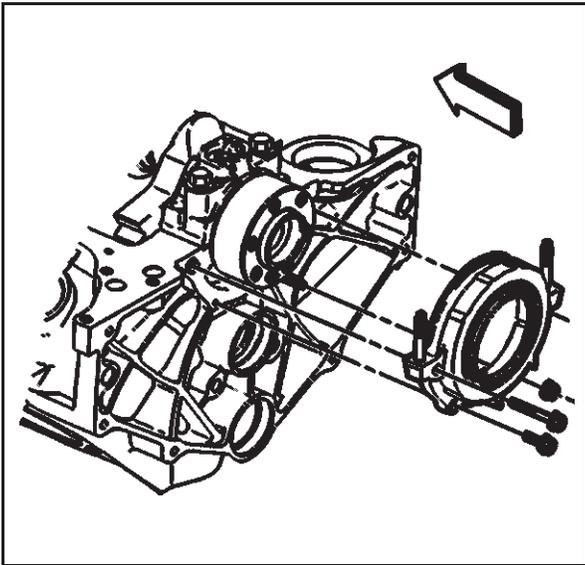
4. Remove the crankshaft rear oil seal housing nut and bolts.
