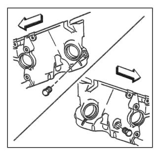
4. Remove both the engine block coolant drain hole plugs and allow the coolant to drain into a suitable container.
