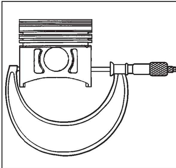
3. With a micrometer or caliper at a right angle to the piston pin bore, measure the piston 11 mm (0.433 in) from the bottom of the skirt.
