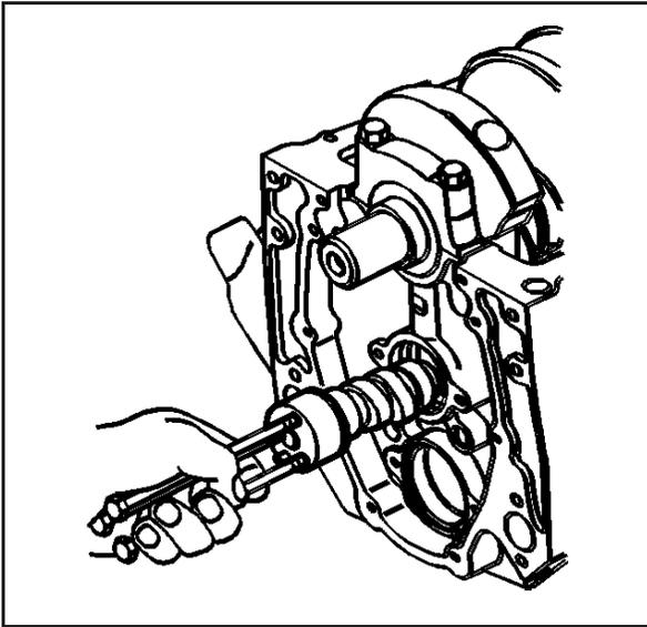
**Notice:** All camshaft journals are the same diameter, so care must be used in removing or installing the camshaft to avoid damage to the camshaft bearings.
