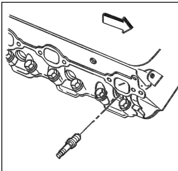
2. Remove the bolts and the spark plug wire support.
