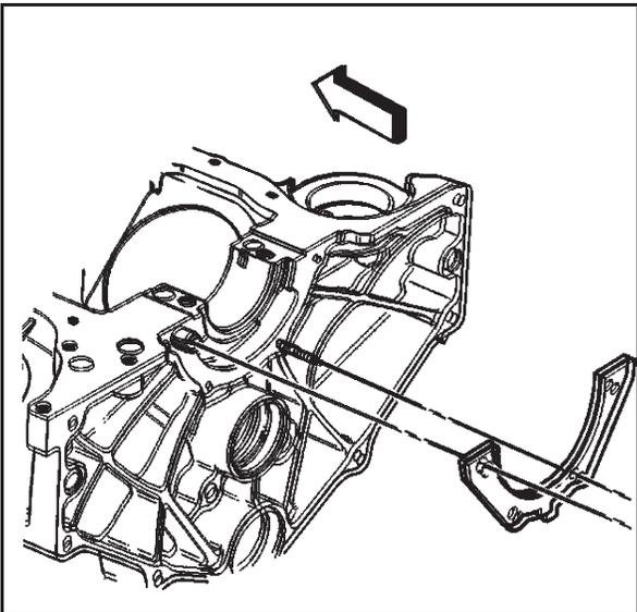
6. Remove the crankshaft rear oil seal housing gasket.
