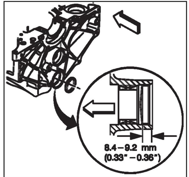
8. Apply Aviation Form-A-Gasket Liquid Sealant or equivalent to the outside diameter of the NEW expansion cup plug (camshaft rear bearing hole).
