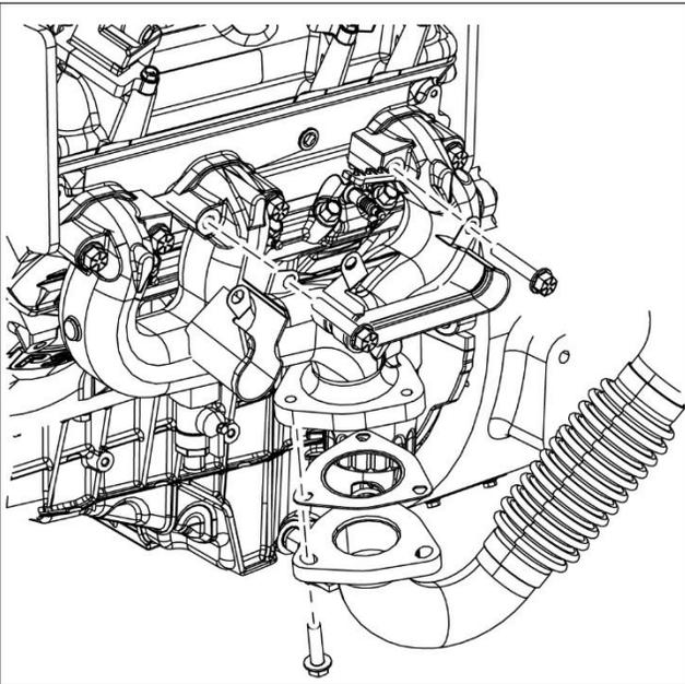
2. Install the exhaust manifold.
