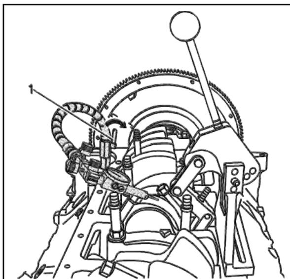
18. Adjust the swivel base as required and position the indicator tip slightly above the connecting rod bolt. Lock the swivel base in position by rotating the locking lever (1). Do not allow the tip of the indicator to contact the connecting rod at this time.
