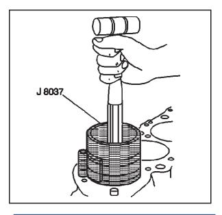
7. Use the J 8037 and the J 5239 and lightly tap the top of the piston with a wooden hammer handle.
