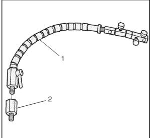
**Important:** The clamp of the swivel base and the shaft of the indicator should be free of oil or other debris. A loose or improperly clamped indicator may indicate incorrect readings.
