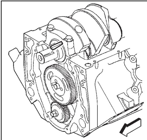
6. Remove the crankshaft balancer key.
