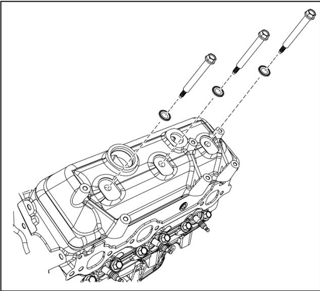
3. Install the valve rocker arm cover onto the cylinder head.
