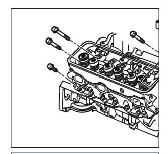
10. Tighten the cylinder head bolts in sequence on the first pass.
