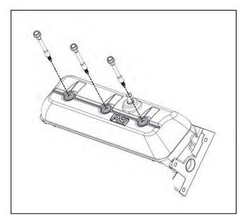
4. Install the valve rocker arm cover bolts.
