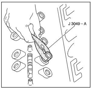
**Important:** Some valve lifters may be stuck in the valve lifter bores because of gum or varnish deposits and may require the use of J 3049-A for removal.
