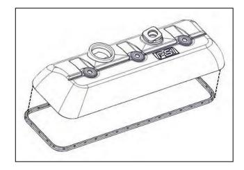
3. Install the valve rocker arm cover onto the cylinder head.
