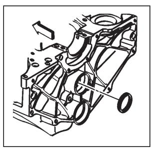
6. Remove the expansion cup plug (camshaft rear bearing hole) and discard.
