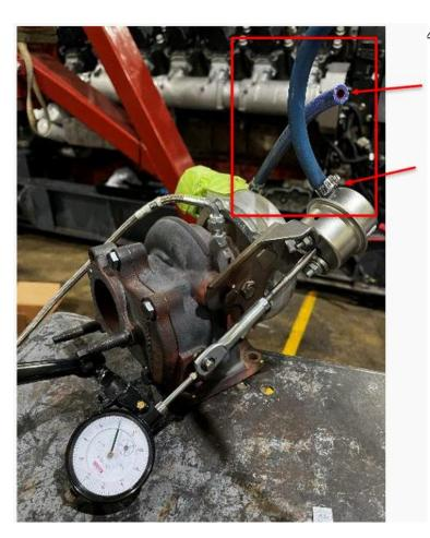
Disconnect the hose currently attached to the actuator, and then connect the hose from the pressure regulator setup directly to the actuator.
