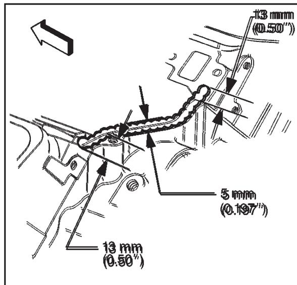
4. Apply a 5.0 mm (0.197 in) bead of UltraGray RTV or equivalent to the rear top of the engine block.
