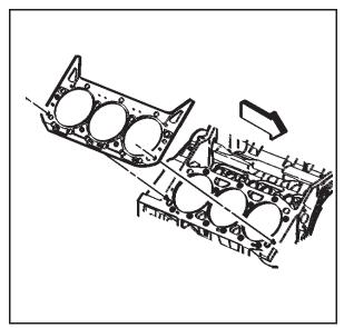
**Important:** Do not use any type of sealer on the cylinder head gasket (unless specified).
