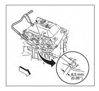
4. Install the oil level indicator into the oil level indicator tube, if required.
