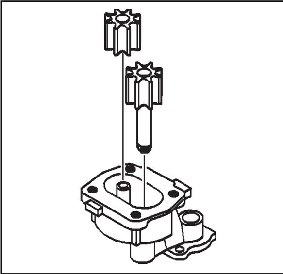
5. Remove the oil pump drive gear and the oil pump driven gear.
