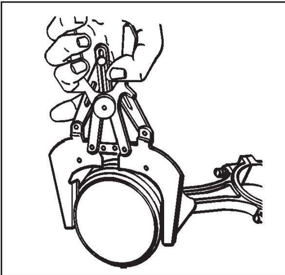
3. Clean the piston ring grooves with a suitable ring groove cleaning tool.
