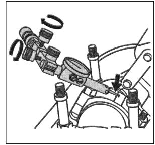
21. Lightly actuate the handle of the pivot arm assembly (multiple times in both directions) to ensure the oil film is removed from the journal.
