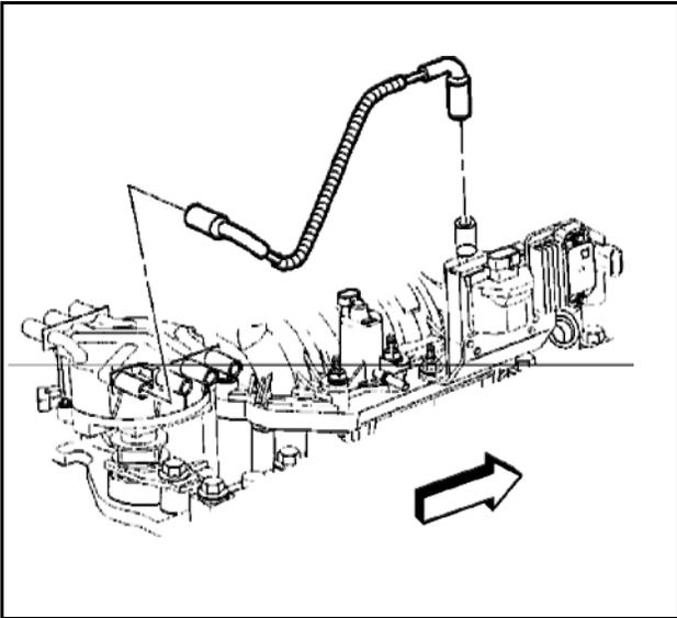
2. Remove the distributor clamp bolt.
