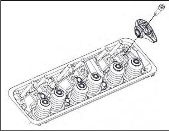
2. Remove the valve pushrods.
