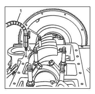
17. Install the swivel base (1) to the oil pan rail of the engine block. Tighten until snug.
