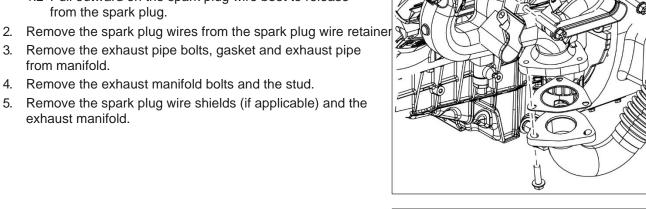
6. Remove and discard the exhaust manifold gaskets.
