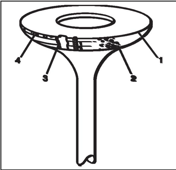
6. Inspect the valve contact surface for the following:
