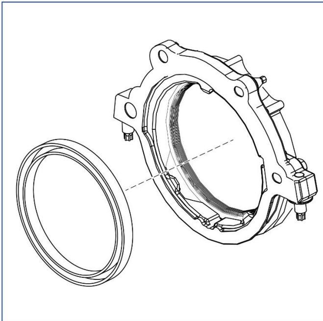
10. Remove the sleeve from the crankshaft rear oil seal.
