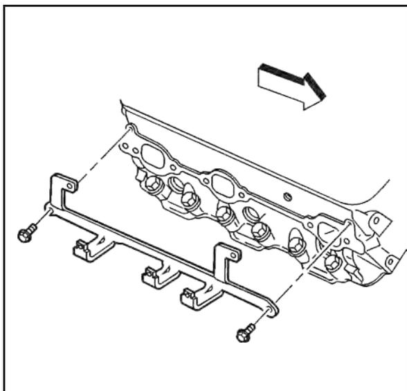
3. Remove the cylinder head bolts and discard.
