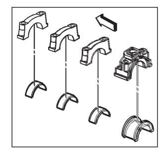
7. Install the crankshaft bearing caps in the original position and with the arrow on the crankshaft bearing caps in the direction of the front of the engine block.
