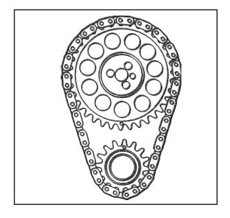
6. Look to ensure that the crankshaft sprocket is aligned at the 12 o'clock position and the camshaft sprocket is aligned at the 6 o'clock position.
