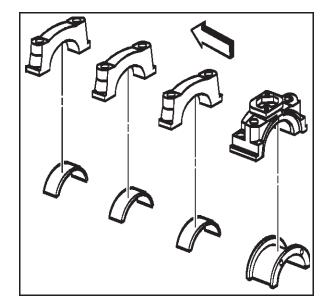
5. Install the crankshaft bearing caps in the original positions and with the arrow on the crankshaft bearing caps in the direction of the front of the engine block.
