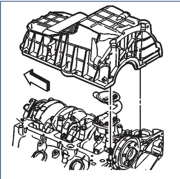
**Important:** The oil pan alignment must always be flush or forward no more than 0.3 mm (0.011 in) from the rear face of the engine block.
