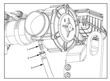
2. Loosen hose clamp (2) and slide back on hose (3), remove hose (3) from fitting (1).
