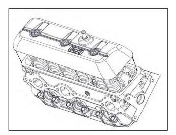
4. Remove the valve rocker arm cover.
