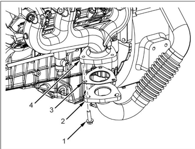
7. Install left side turbo exhaust (2) and new gasket (3) to left side exhaust manifold (4) and secure with bolts (1).
