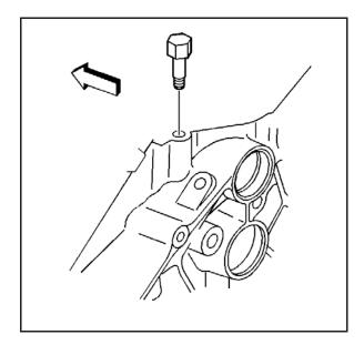
3. Remove the dowel straight pins
