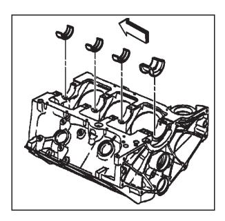
6. Remove the crankshaft bearings from the engine block.
