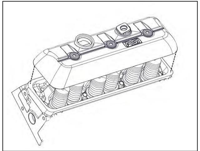
5. Remove the valve rocker arm cover gasket.
