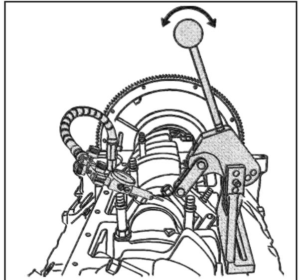
22. Load the handle in the forward position and zero the dial indicator. Load the handle multiple times in both directions and record the reading.
