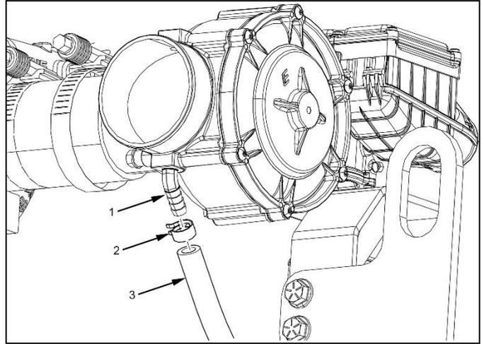
2. Loosen hose clamp (2) and slide back on hose (3), remove hose (3) from fitting (1).
