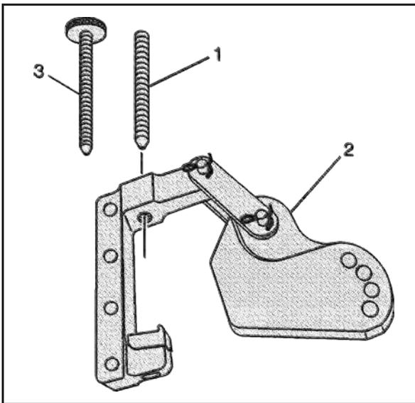
6. Install the screw (1 or 3) to the pivot arm assembly (2).
