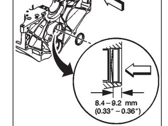
Apply PTFE Sealant or equivalent to the threads of the engine block left side oil gallery plug. Located above oil filter housing.
