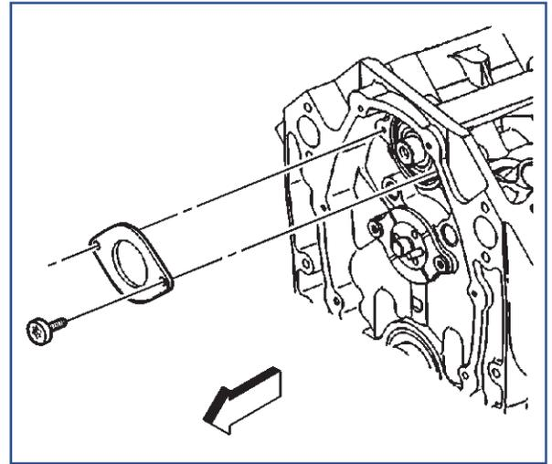
Install the balance shaft driven gear onto the balance shaft.
