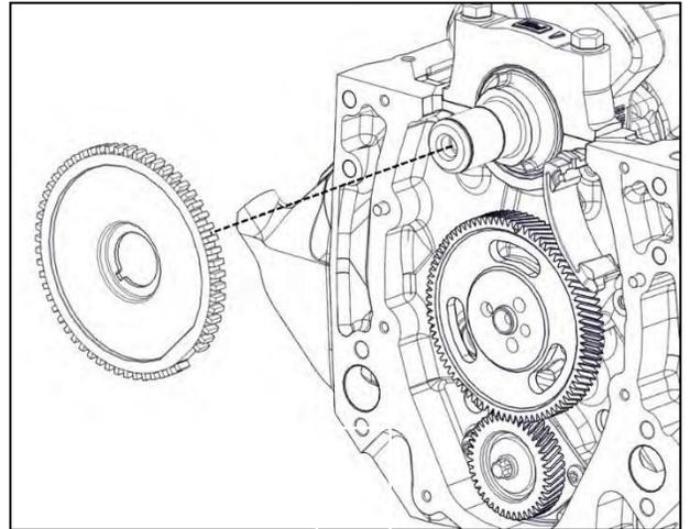
**Camshaft Sensor Installation; Coil Near Plug (CNP)**
