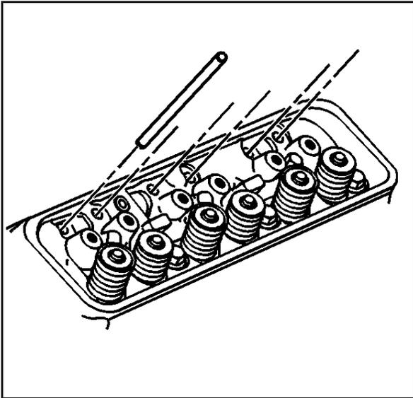
**Valve Rocker Arm and Push Rod Installation**
