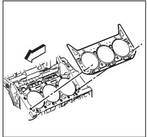
Install the cylinder head onto the engine block.
