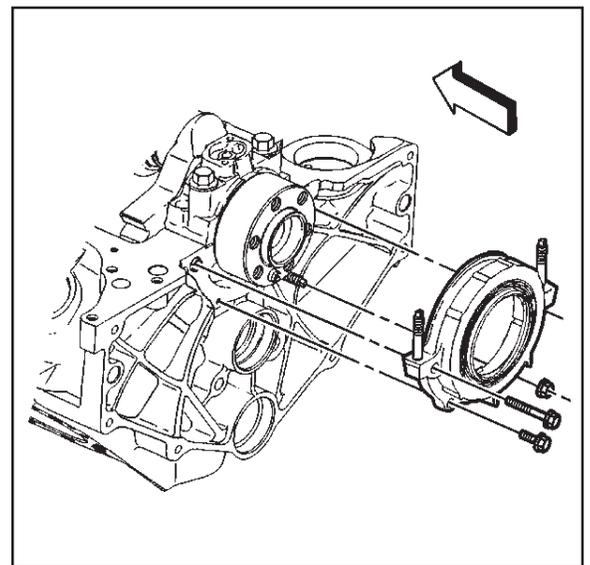
5. Apply a small amount (2 to 3 drops) of clean engine oil to the bore of the crankshaft rear oil seal housing.
