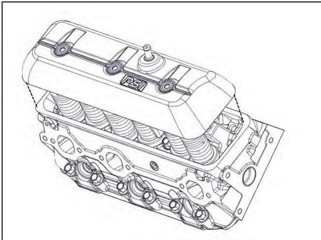
3. Install the valve rocker arm cover onto the cylinder head.
