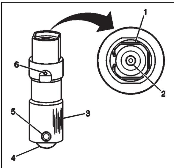
6. Inspect the valve lifter for the following:
