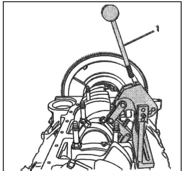
15. Select the adapter (2) (as required) and install to the swivel base (1). Tighten until snug.
