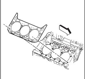
6. Remove the dowel pins (cylinder head locator) (if required).
