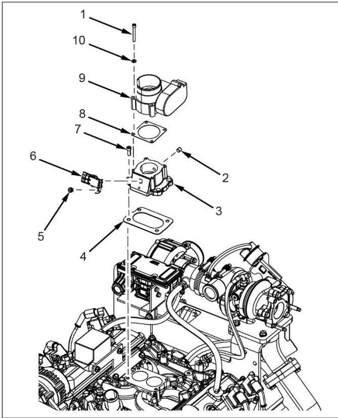
6. Remove bolt (5) and T-Map sensor (6) remove sensor from intake adapter (6).
