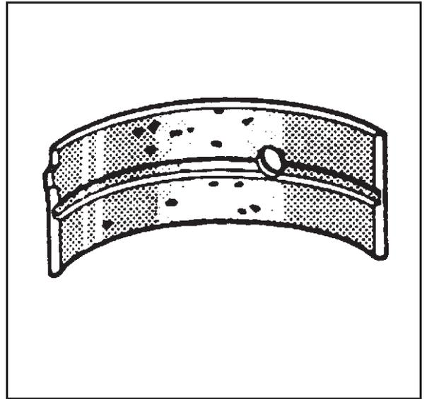
12. Inspect the crankshaft bearings for excessive scoring or discoloration.
