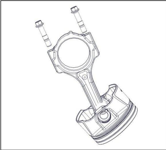
**Important:** The mark on the top of the piston • must face the front of the engine block.
