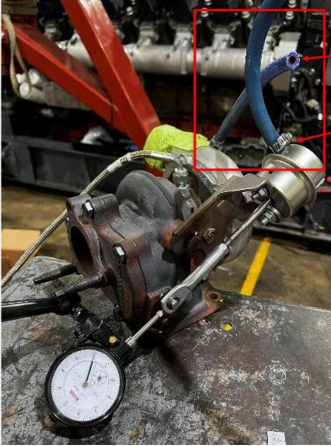
4. Disconnect the hose currently attached to the actuator, and then connect the hose from the pressure regulator setup directly to the actuator.
