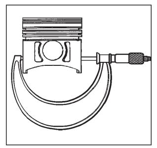
15. Measure the piston with a micrometer at a right angle to the piston pin bore, measure the piston at 11 mm (0.433 in) from the bottom of the skirt. Refer to *Engine Mechanical Specifications*.
