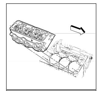
5. Remove and discard the cylinder head gasket.
