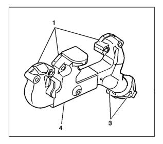
4. Measure the alignment or surface flatness of the exhaust manifold flanges using a straight edge and a feeler gauge. Refer to *Engine Mechanical Specifications*.
