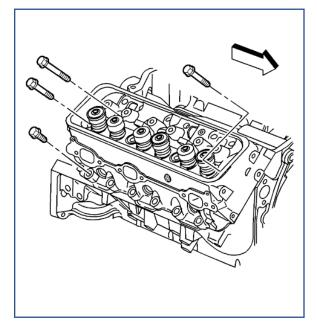
3. Remove the cylinder head bolts and discard.
