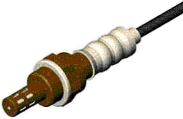
The Heat Exhaust Gas Oxygen (HEGO) Sensor HEGO1 (upstream or before the catalytic converter) and HEGO2 (downstream) voltage output.
