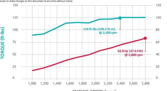
**ENGINE SPEED (rpm)**
